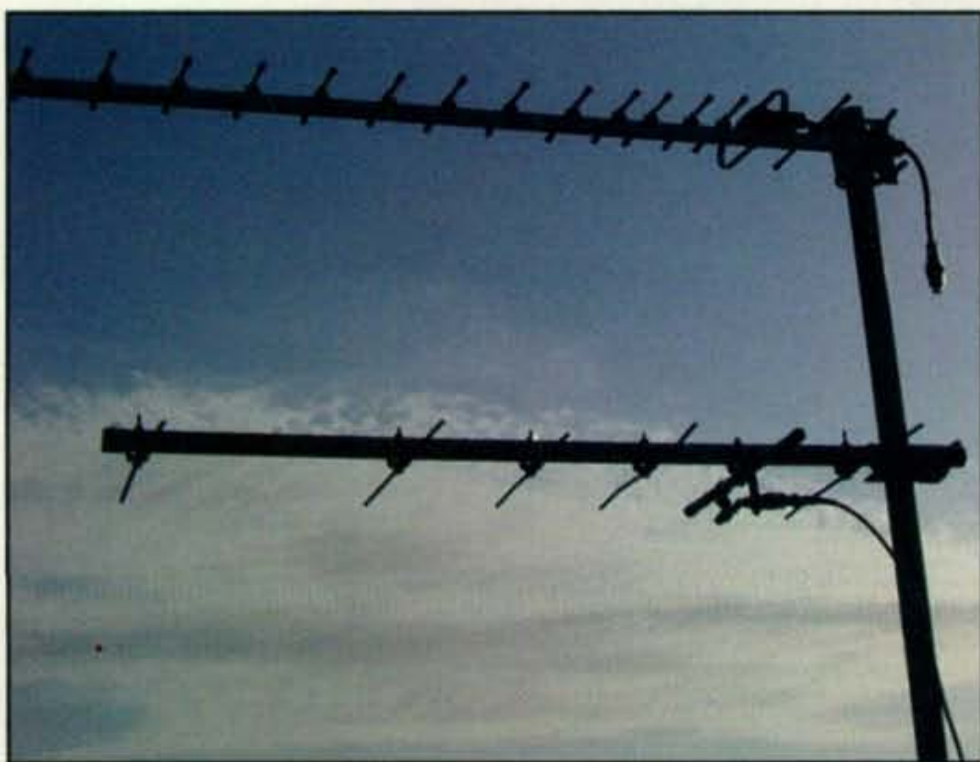
Photo A— Measuring a 440-MHz Yagi and its interaction with a 915-MHz Yagi.
